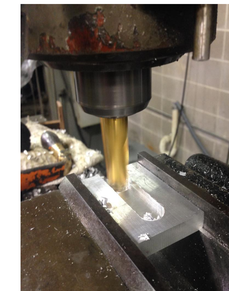
Milling of Components
