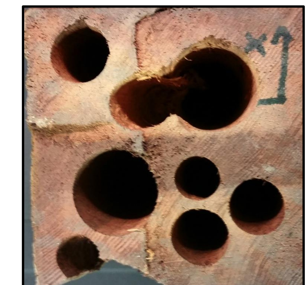
Figure 3: Swiss Cheese Defect Test Sample
